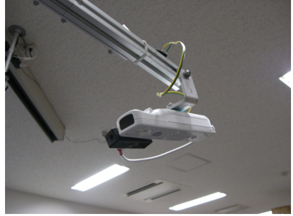
Figure 6. IR camera for pen recognition
